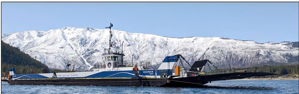
Figure 4-18: Example of Cable Ferry with a 24-Vehicle Capacity in British Columbia, Canada
